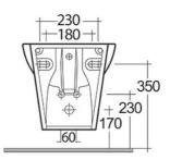
Dimensions: All dimensions in mm tolerance ±5% for below 200mm and ±3% for above 200mm. Note: Due to a continuing development programme to improve design and performance, the manufacturer reserves all rights to vary specifications without prior information. Please note accessories are for photographic use only.
